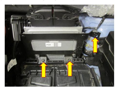
4. The battery tray is the next component that needs to be removed, to do this remove the three 12mm fasteners holding the battery tray to the chassis, use a 12mm socket with extension bar to do this. There is also a wiring harness attached to the battery tray which is held in place with two 10mm fasteners, remove both fasteners with a 10mm socket and rachet to release the wiring loom. Now lift the tray from the engine bay.
