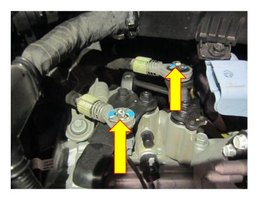
6. There are three 14mm fasteners that hold the linkage to the gearbox. Remove these with a 14mm socket and rachet, with these removed the linkage will lift off with gentle persuasion.
